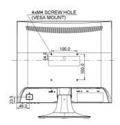
All trademarks and registered trademarks acknowledged. E & O E. Specification subject to change without notice. All LCD's comply with ISO-9241-307:2008 in connection with pixel defects.
